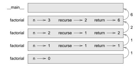
The return values are shown being passed back up the stack. In each frame, the return value is the value of result, which is the product of n and recurse.
