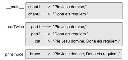
The order of the stack shows the flow of execution. printTwice was called by catTwice, and catTwice was called by \_main\_, which is a special name for the topmost function. When you create a variable outside of any function, it belongs to \_main\_.
