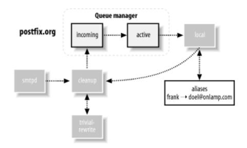
Figure 3-5. Tracing message delivery 2
