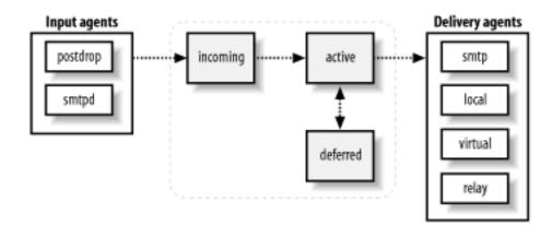
From the incoming queue, the queue manager moves messages to the active queue and invokes the appropriate delivery agent to handle them. For the most part, if there are no problems with delivery, movement through the queue is so fast that you won't see messages in the queue. If Postfix is trying to deliver to a slow or unavailable SMTP server, you may see messages in the active queue. Postfix waits 30 seconds to decide if a remote system is unreachable.
